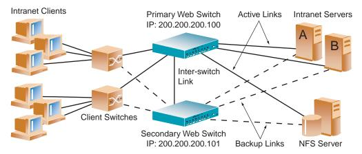
**Figure 11-3** A Non-VRRP, Hot-Standby Configuration
